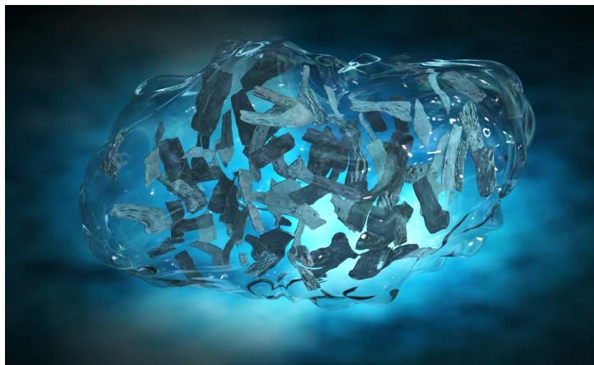
Fig. 1. NanoBone consist of nanocrystals of hydroxyapatite, the same mineral as bone, and an amorphous silica matrix.
